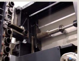
Consistent tool change operation and superior durability are ensured by use of the acknowledged OKK's original cam-controlled high-speed synchronizing tool changer (OKK
