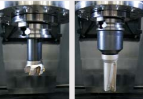
φ63.0 (2.48") Side cutting for shoulder φ50.0 (1.97") Drill
