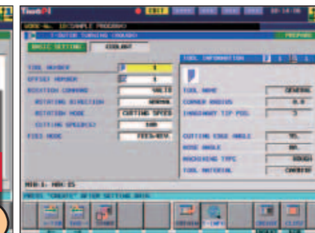
In case of new work piece Programming, number of input items are much less due to automatic cutting data setting.
