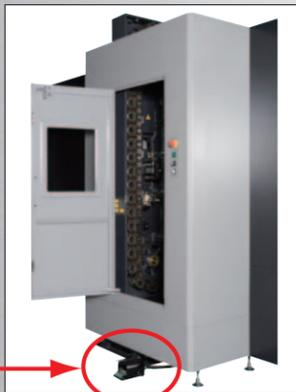
Foot-operated switch for removing a tool (Standard)
