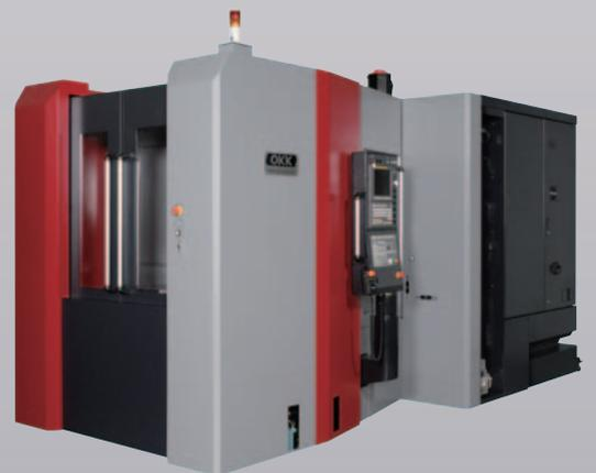
This high-speed machine features the strongest structural rigidity in its class and attains a rapid feed rate of 63m/min(2480ipm) with 1G acceleration.
